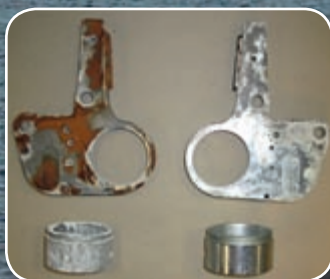
The tools are also salt spray tested.
