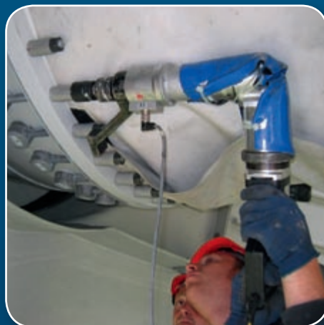
Measurement Transducer KBW mounted on the DEMW (90° angle drive)
